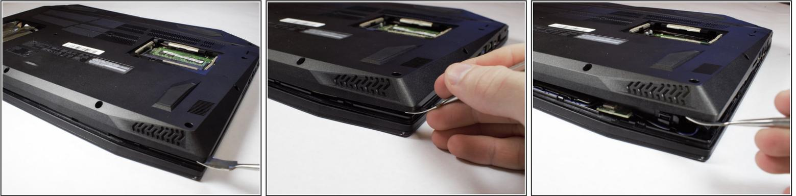
**⚠ Be sure you removed the hard drive.** when you open the back shell and hard drive is built in this may cause damage to cable and other components.
