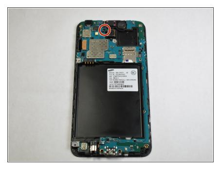
Remove single screw from back of device. This is the only screw that must be removed to take off this piece.
