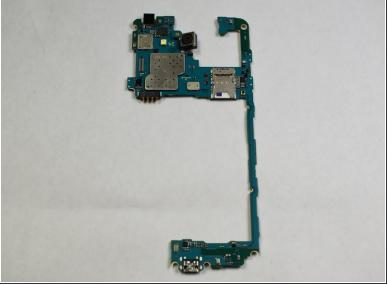
• Pull the blue/green piece away from the black piece. They should not need any force to be removed. The next step will deal with using the green/blue piece from the second picture.
