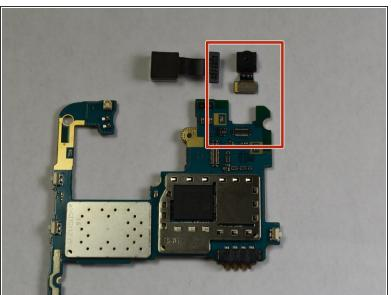
Flip over the piece (180 degrees). Remove the boxed out piece. This is the front facing camera.
