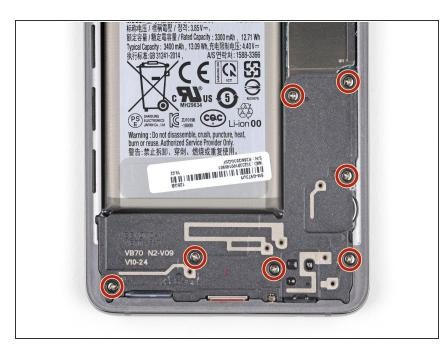
Remove the seven 4 mm Phillips screws securing the lower midframe.
