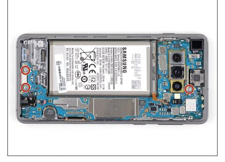
Remove the three 3.7 mm Phillips screws securing the motherboard to the phone.
