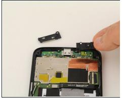
Unscrew four 1.8mm T4 screws from the speakers and remove from the motherboard.
