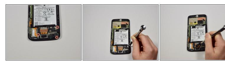
Unscrew the three 1.7mm T4 screws from the speaker.
