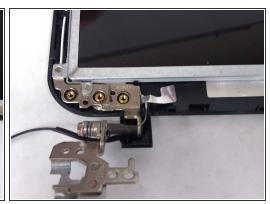
Remove the three 4.1 mm Phillips #0 screws attaching each hinge to the screen.
