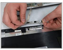
Once the screen has been detached and turned over, remove the webcam from its place on the bezel.
