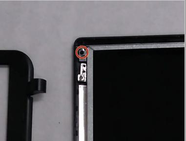
• Remove the two 3.1 mm Phillips #0 screws at the top of the screen.
