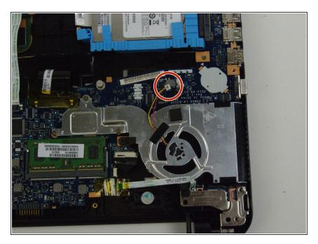
Disconnect the fan wire from the motherboard.
