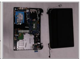
Pivot and lift up the monitor and separate it from the base of the laptop.
