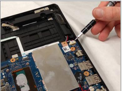
• As in Step 8, gently pry out both sides of the white connector and pull out the connector.
