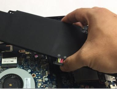
Once the screws and connector are removed, simply pull out the battery from its place.
