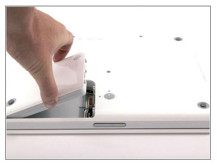
Lift the battery out of the computer.
