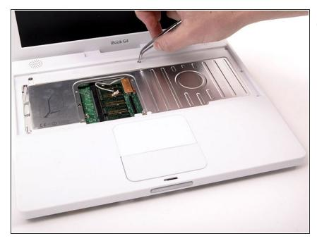
We recommend placing the computer on a slab of grey antistatic packing foam from this point on to prevent damaging the logic board.
