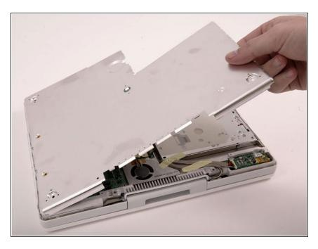
Lift the bottom shield off.
