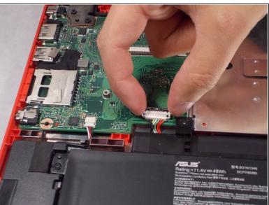
• Using your thumb and index finger, pinch the multi-color cable and disconnect it from the motherboard.
