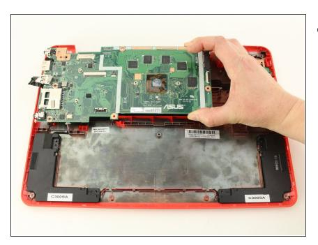
Wiggle and pull the motherboard out from the bottom case.
