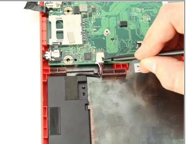
Using the black nylon spudger, carefully slide the speaker cable connector out from its attachment on the motherboard.
