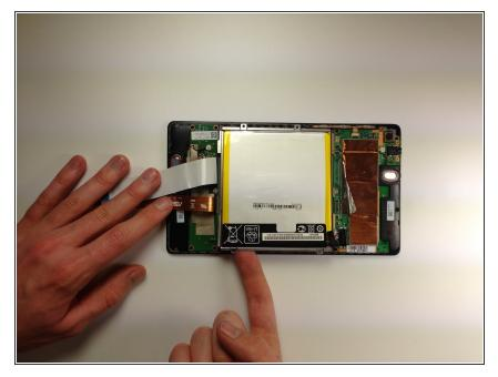
Remove the battery from your device by applying pressure at the base of the battery and lifting it out.
