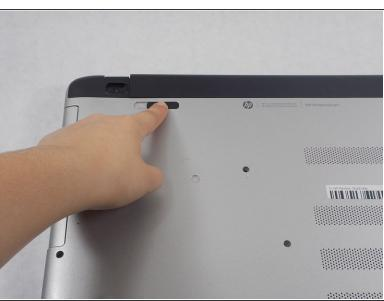
Slide the battery lock (the switch at the upper left corner of the laptop's underside) to the right until it clicks into place.
