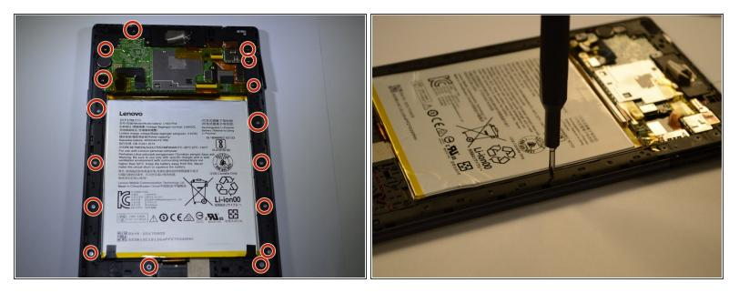
• Remove 16 screws from the midframe with Phillips #000 screwdriver [bit].
