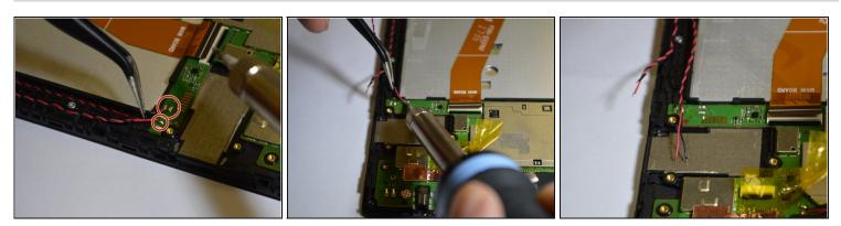
• Desolder the black and red speaker wires from the motherboard.
