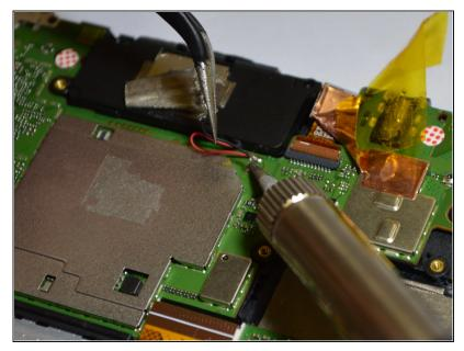
• <u>Desolder</u> the two top speaker wires from the motherboard.
