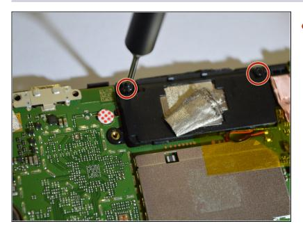
• Use a Phillips #000 screwdriver to remove the two screws that secure the speaker to the motherboard.
