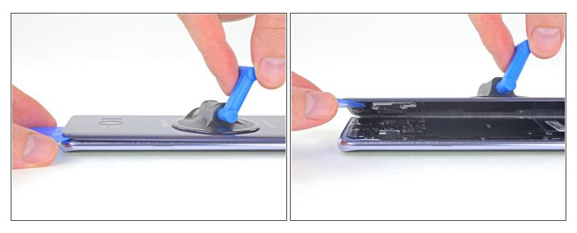
$\bigwedge$  Don't try to fully remove the back cover yet.
