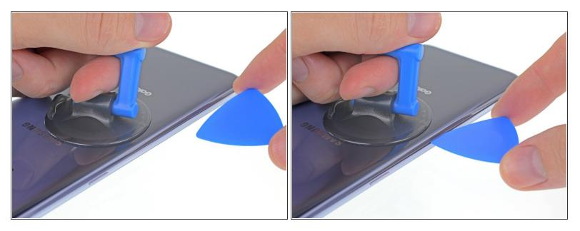
Insert an opening pick into the gap.
