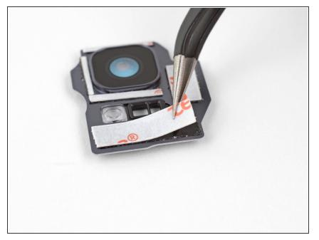
Use tweezers to peel the backing off all the adhesive on the rear camera bezel.
