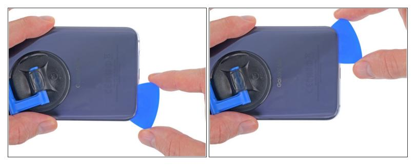
• Continue slicing through the adhesive along the bottom edge of the phone.
