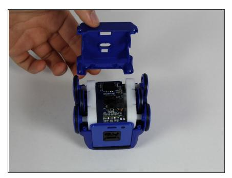
Carefully remove the bottom panel of the Spin Master Boxer by lifting up, away from the main body of robot.
