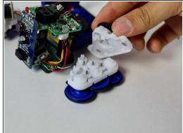
Grip wheel, and gently pull up, to separate white gear casing into its front and back panel.
