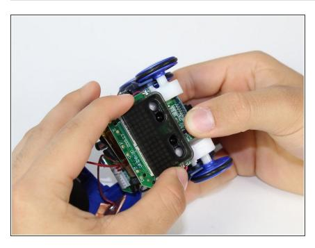
Remove the plastic screen from the body of the robot. It should come off easily as it is not attached by anything.
