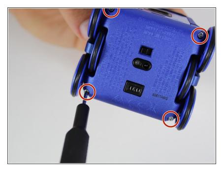
Using a Phillips #00 screw driver, unscrew the four 4mm screws in each corner of the bottom panel.
