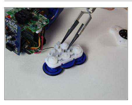
Using tweezers, grip defective gear, and pull up and out of gear system to replace.
