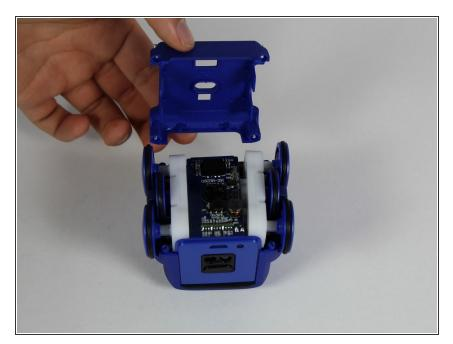
Carefully remove the bottom panel of the Spin Master Boxer by lifting up, away from the main body of robot.
