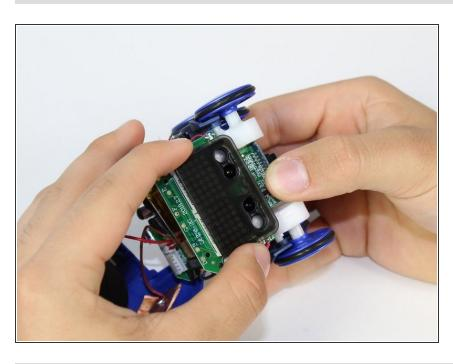
Remove the plastic screen from the body of the robot. It should come off easily as it is not attached by anything.
