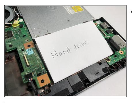
Disconnect the ZIF connector and lift the hard drive out of the space.
