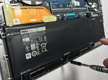
• Using a Phillips #0 screwdriver, remove the seven 3.5mm screws that secure the battery to the palm rest assembly.
