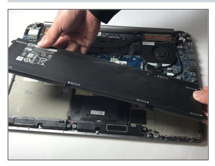
• Lift the battery off the chassis.
