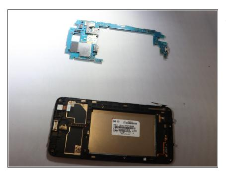
Use the spudger to pry off the motherboard from the rest of the device on the top left corner down to the bottom right corner
