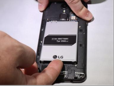
Use the slot in the middle of the bottom edge of the battery to pry it up and out of the case.
