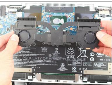
Slide the fan assembly toward you, and when the top edge of the fan is out of the vent grill, the fan is completely removed.
