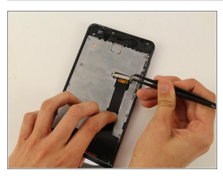
Remove the metal bracket with a tweezer.
