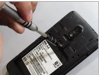
Unscrew the 13 Phillips #0 screws from the back of the phone.
