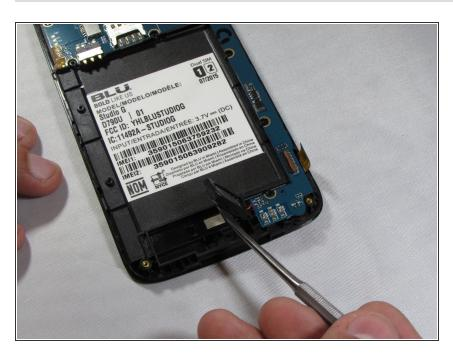
Locate the speaker on the bottom of the device and slowly pry upwards and to the right as its wired to the motherboard.
