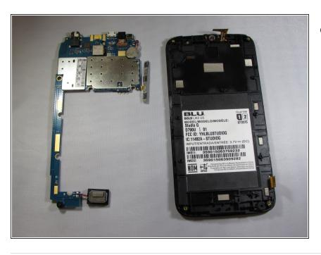
The antennae will be soldered directly to the motherboard which will be replaced.
