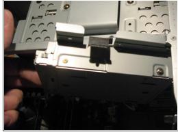
To remove Floppy drive, Unlatch Retainer and swing Drive outward as shown.
