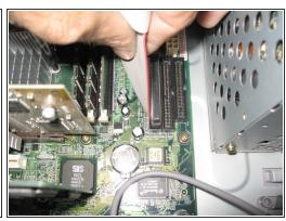
Then Remove the other end of the IDE cables from the Motherboard
