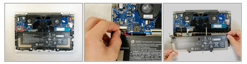
• Carefully remove the power supply connector by pulling on both sides of its head.
