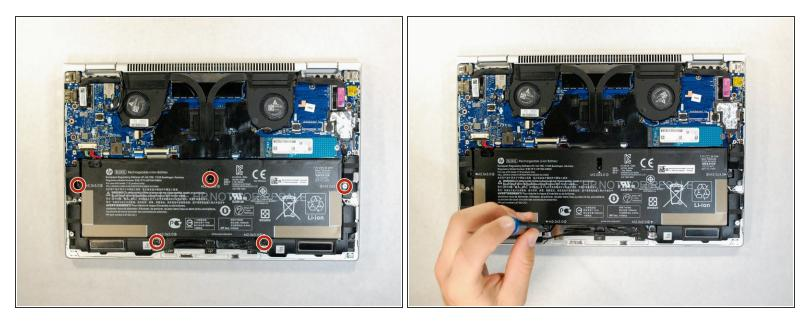
• Use the Phillips 1 screwdriver to remove the five 3mm Phillips screws from the battery assembly.
