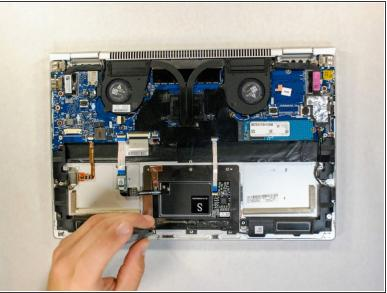
• Use the Phillips 0 screwdriver to remove the six 3mm Phillips screws from the touchpad assembly.
