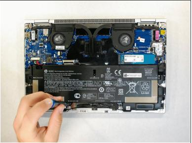
Use the Phillips 1 screwdriver to remove the five 3mm Phillips screws from the battery assembly.
