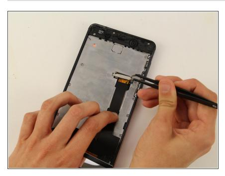
Remove the metal bracket with a tweezer.
