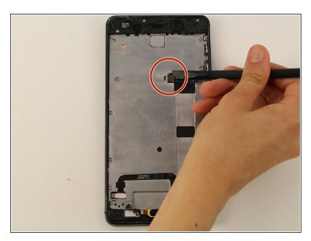
Disconnect the battery connector with a spudger.
