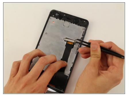
• Remove the metal bracket with a tweezer.
