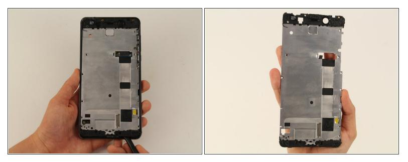
• Decouple the midframe with the spudger and remove the midframe from the device.
