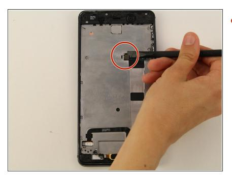
Disconnect the battery connector with a spudger.
