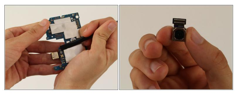
• Remove the 8MP front-facing camera with the spudger.
