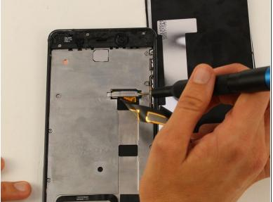
Use a Phillips #000 screwdriver to remove the 1 mm x 1.4 mm screw holding down the metal bracket over the screen ribbon connector.
