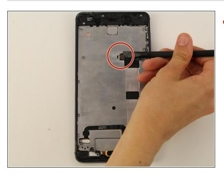
Disconnect the battery connector with a spudger.
