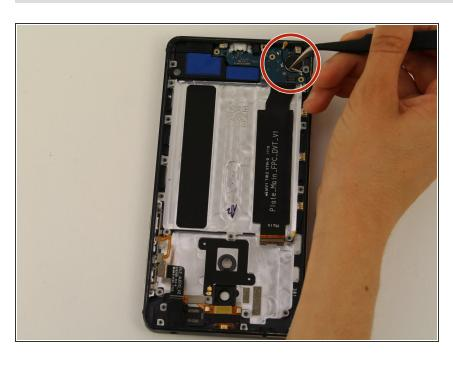
With tweezers, lift the wire by the microUSB port and the microphone unit.
