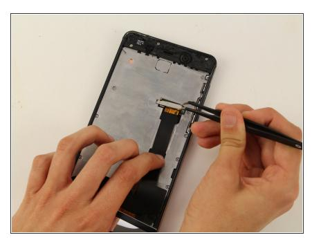
Remove the metal bracket with a tweezer.
