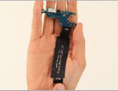
• Remove the microUSB port and the microphone by lifting the unit with a spudger.
