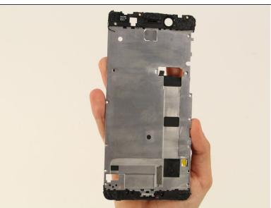
Decouple the midframe with the spudger and remove the midframe from the device.
