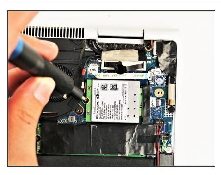
Remove the 2.4 mm screw holding the card down using a Phillips #00 screwdriver.
