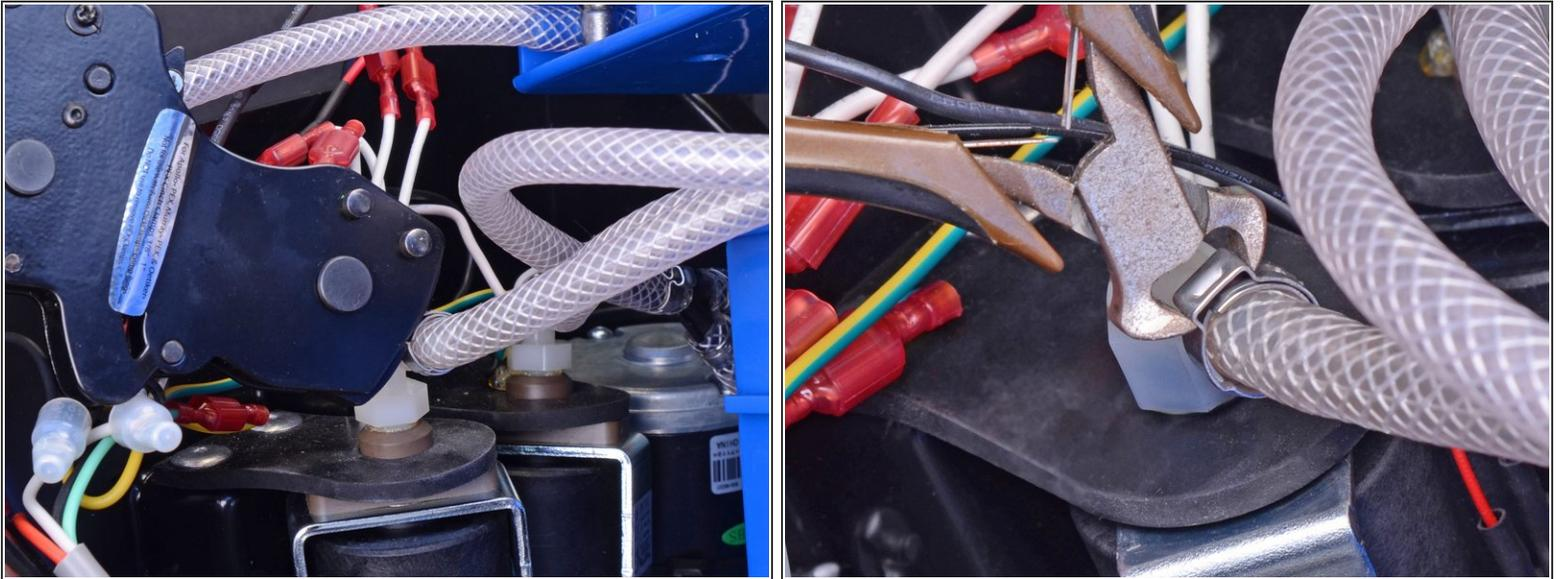
✦ **Re-assembly tip**—to reinstall the crimp-style hose clamps:
