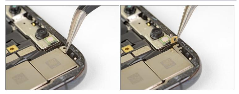
• Use tweezers to gently fold the small metal grounding bracket out of the way. Do not pull up on it as it is connected to a fragile flex cable.
