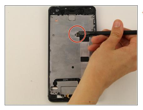
Disconnect the battery connector with a spudger.
