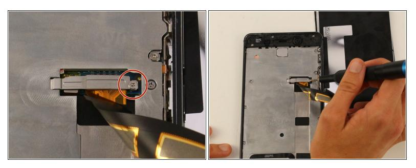
• Use a Phillips #000 screwdriver to remove the 1 mm x 1.4 mm screw holding down the metal bracket over the screen ribbon connector.
