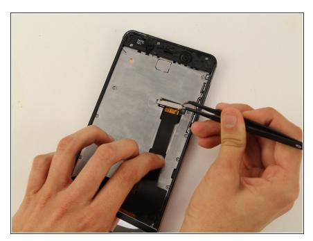
Remove the metal bracket with a tweezer.
