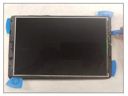
Continue along the outer edge of the housing until you have placed an iFixit opening pick in each corner.
