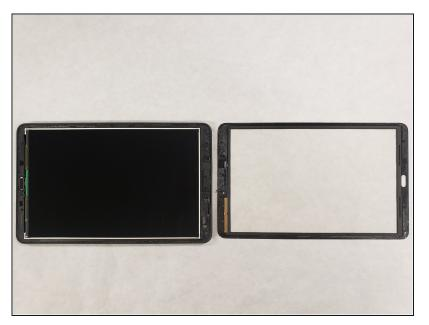
Place the removed screen that is still attached to the ribbon cable flat on the table.
