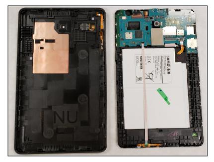
Remove the LCD assembly from the housing and place it face down on the table.
