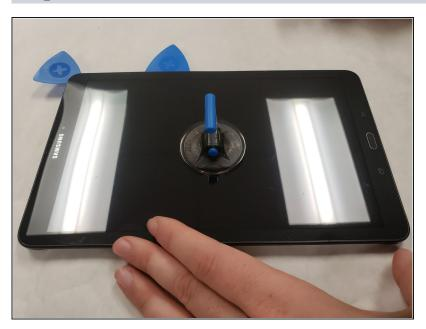
Place the iFixit opening pick between the lifted corner and the housing to prevent the screen from falling back into the housing.
