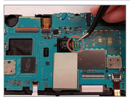
Use the curved precision tweezers and carefully peel off the protective green film on top of the camera connector.
