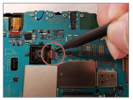
Use the spudger and gently pry the ZIF connector lock tab upwards, releasing the ribbon cable.
