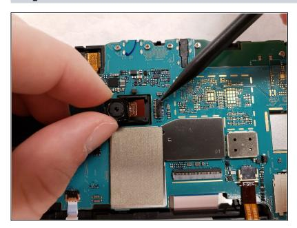
Grab the camera and pull up and away from the connector.
