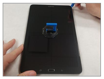
Grab the iFixit opening tool and wedge the sharp end into the corner of the screen. Pry it upwards, lifting up the corner of the screen.
