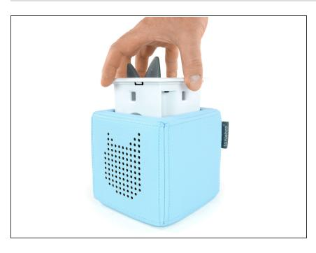
Lift the inner part out of the foam housing.
