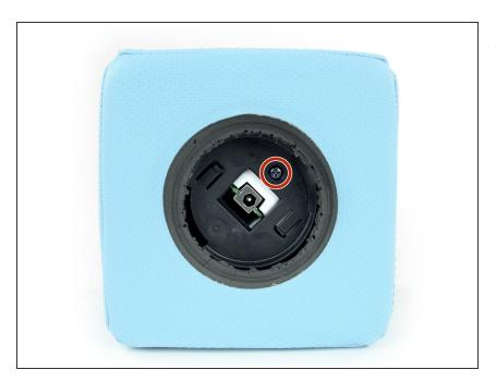
Remove the Phillips #1 screw on the bottom of the Toniebox.
