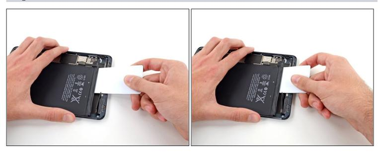
• Remove the card and reinsert it, beneath the bottom right corner of the battery.
