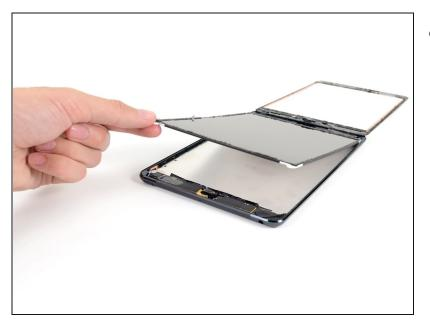
• Lift the LCD up a couple inches from the rear case to ensure it's free from the adhesive.
