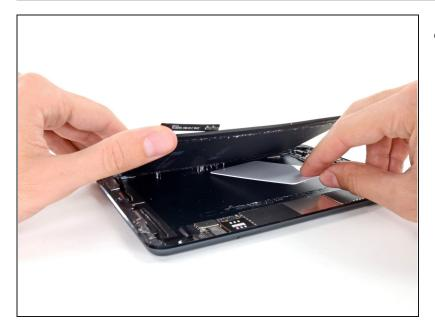
• While lifting the right side of the battery up with one hand, use a plastic card to cut any adhesive still holding the battery down to the rear case.
