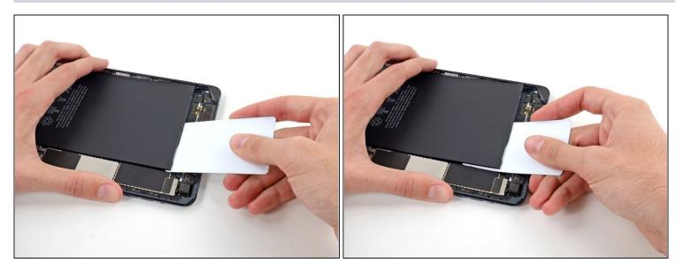
• Remove the plastic card and reinsert it underneath the top right corner of the battery.
