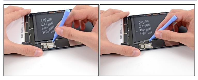
• Use a plastic opening tool to gently pry the battery connector up from its socket on the logic board.
