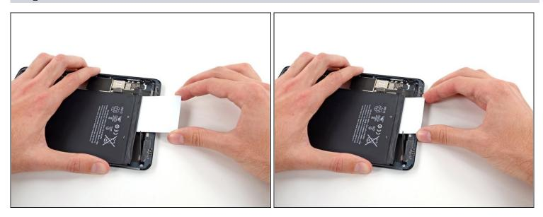
• Push the card further underneath the battery.
