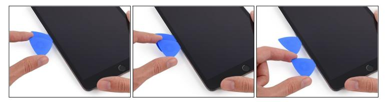
• Place a second opening pick alongside the first and slide the pick down along the edge of the iPad, releasing the adhesive as you go.
