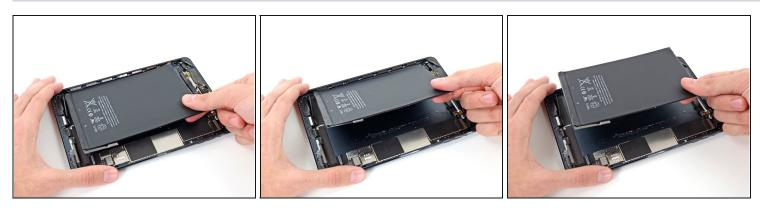
• Lift and remove the battery from the iPad.
