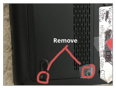
Remove the two screws on the hard drive lid
