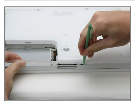
• Run a spudger along the seam between the lower case and upper case on the front of the computer to free the tabs locking the lower case. Pull up on the lower case and continue to use the spudger as necessary until you hear three distinct clicks.
