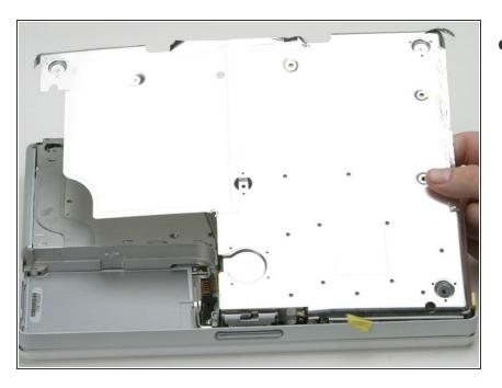
Lift the bottom shield off.
