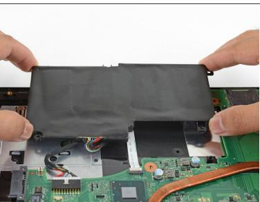
Lift the battery out of its recess and move it slightly away from the motherboard in order to reveal the battery cable.
