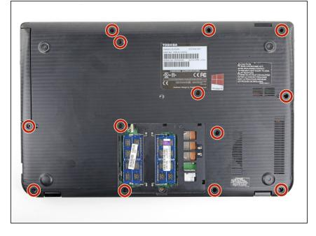
Remove the thirteen 6.8 mm long Phillips screws securing the back cover.
