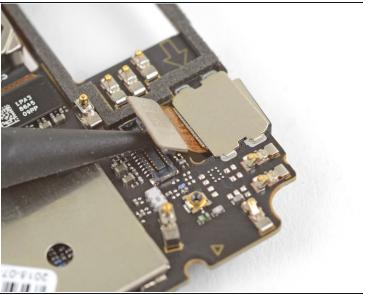
• Use the point of a spudger to pry up and disconnect the front-facing camera from its motherboard socket.
