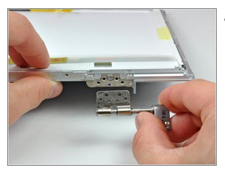
Remove the left clutch hinge from the front display bezel.
