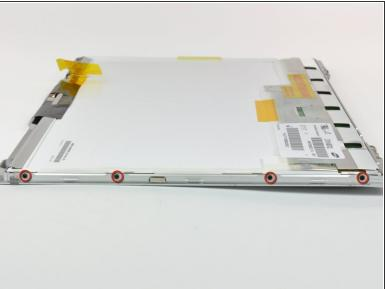
Remove the four Phillips screws from each side of the display (eight screws total).
