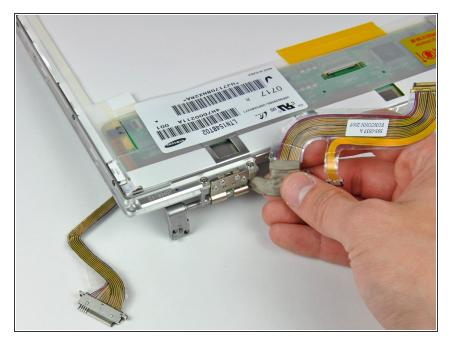
De-route the display data cable from the right clutch hinge and set it aside.
