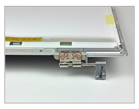
Remove the four T6 Torx screws securing the left clutch hinge to the front display bezel.
