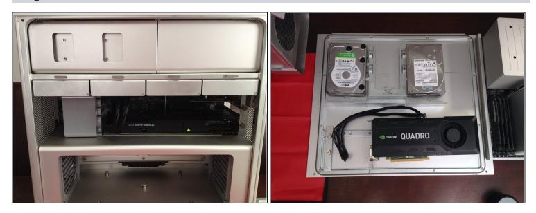
• Remove the hard disks and the video card from the computer. Put them on the lid, out of the way. Also remove the video card power cables.
