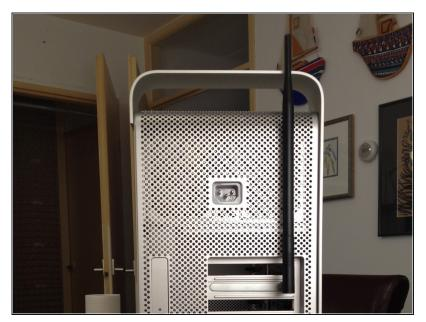
Finally the antenna can be screwed onto the outside of the PCIe slot cover.
