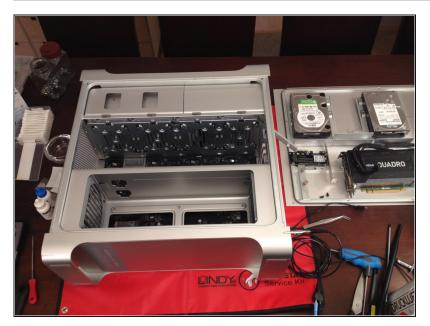
Lay the Mac Pro on its side for more convenient access to the Blue Tooth device.
