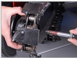
Support the chain roller assembly with one hand while you remove the bolt holding it in place.
