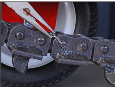
Pull the cotter pin out of the chain pin.
