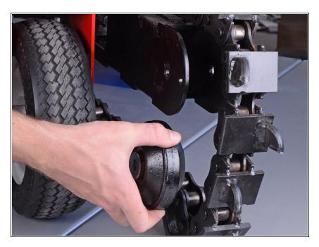
Remove the chain roller assembly.
