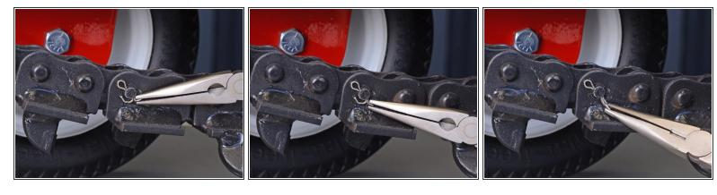
Use a pair of needle-nose pliers to straighten both sides of the cotter pin securing the pin in the master link.
