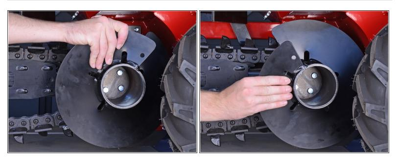
Rotate the auger to move the chain until its master link (the link with the removable pin) is easily accessible.
