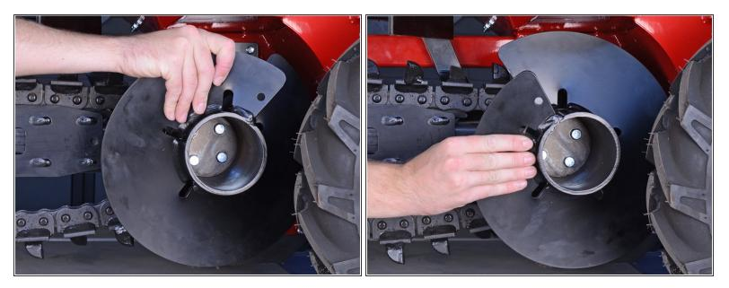
Rotate the auger to move the chain until its master link (the link with the removable pin) is easily accessible.
