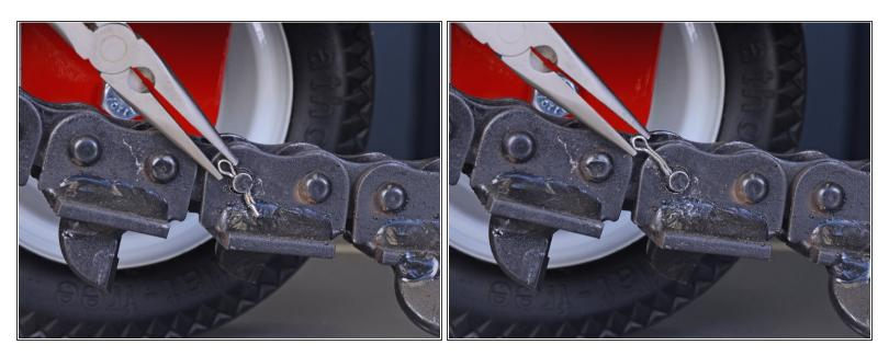
• Pull the cotter pin out of the chain pin.
