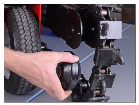
• Remove the chain roller assembly.
