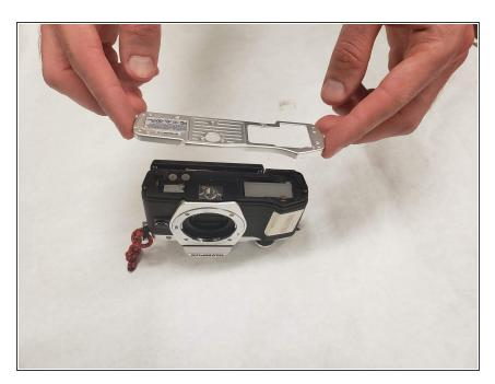
Lift and remove the bottom cover off the camera.
