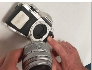
Lay the camera on its back as shown. Using the button located to the right of the lens, hold it down
