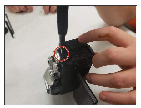
Turn the camera over on its side as shown. There is a small compartment door that has a screw located underneath it. Remove the 2.5 mm screw with a Phillips #00 screwdriver.
