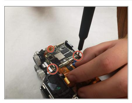
Using a Phillips #00 remove the three 3.0 mm screws while holding the motherboard in place. You should then be able to gently remove the motherboard.
