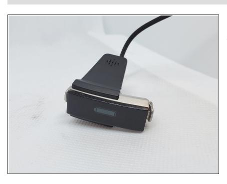
Plug your Fitbit into its charger to turn it back on and charge up the new battery, if needed. Your Fitbit should now hold a charge.
