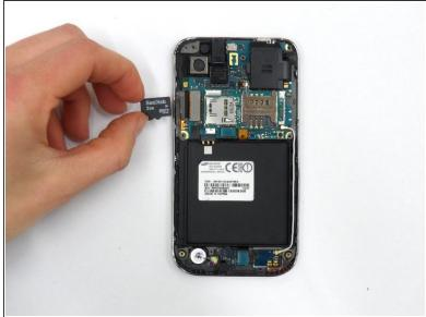
Slide the SD card out of its slot.
