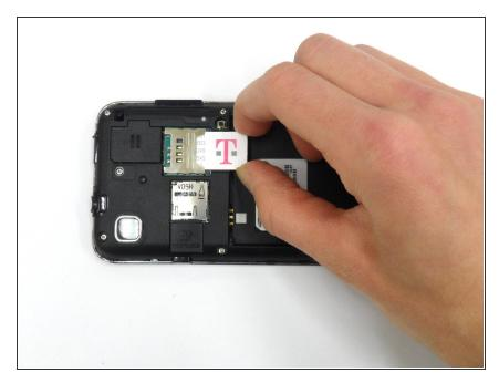
Remove SIM card by pushing down and away from the slot, then pulling it out toward the bottom edge of the phone.
