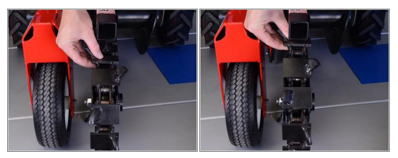
Lift the chain off of the dig sprocket and chain roller and remove it from the trencher.
