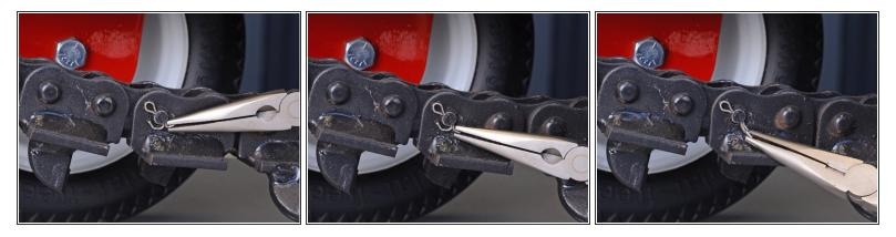
Use a pair of needle-nose pliers to straighten both sides of the cotter pin securing the pin in the master link.
