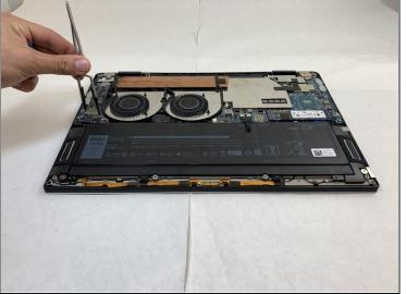
• Use the nylon tweezers to remove the interconnect pins from each of the circuit boards.
